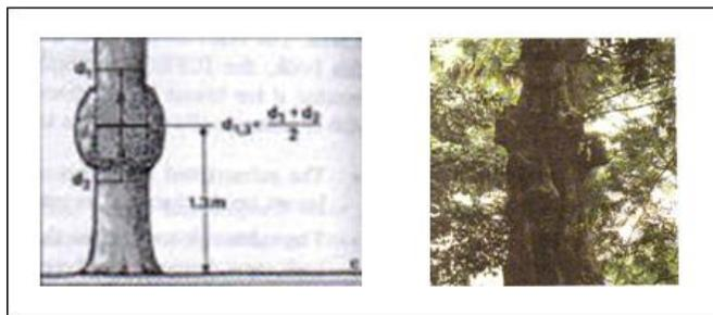
**Gambar 5. Mengukur diameter pohon membengkak**
