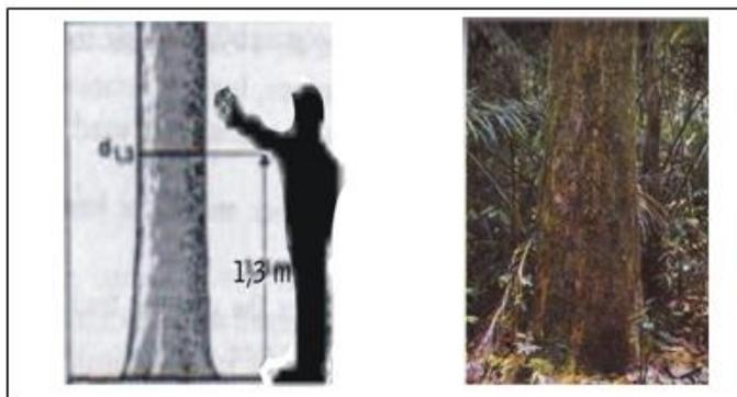
**Gambar 1. Mengukur diameter pohon normal**
