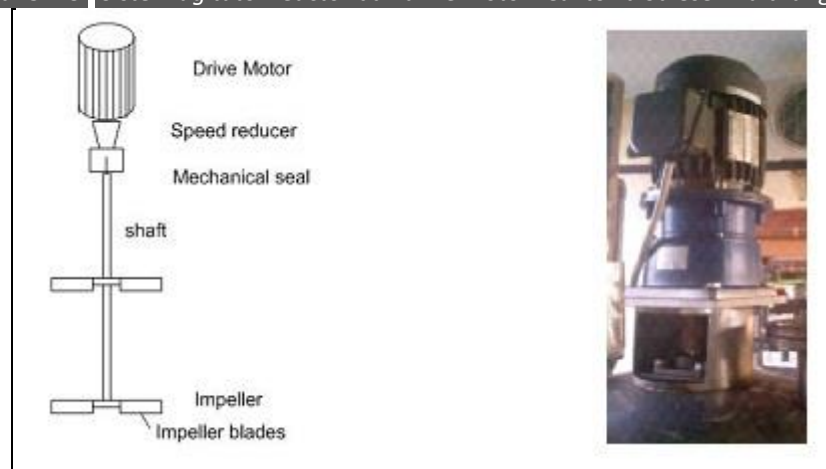
Gambar 5. 23 Sistem agitator reactor dan drive motor reaktor biodiesel multifungsi
