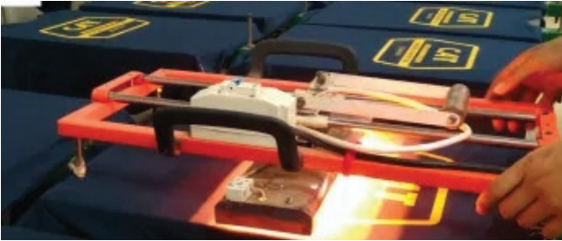
Alat Pengering Curing (Sumber: wizziclothing.com)
