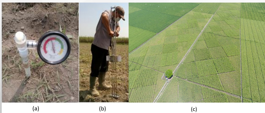
Figure 3 Precision agriculture research measurement activities in Karawang Regency, West Java, Indonesia: a. Soil metric suction measurement; b. Soil penetration measurement; c. Paddy growth monitoring using unmanned aerial vehicle (i.e., UAV drone)
