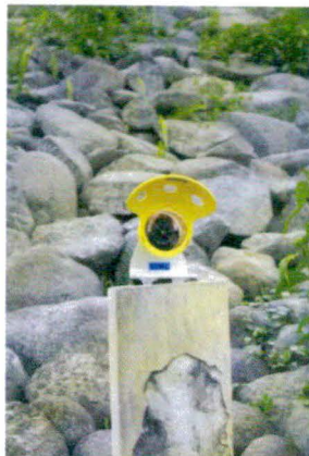
Foto 4.3.1 Prisma target monitoring
