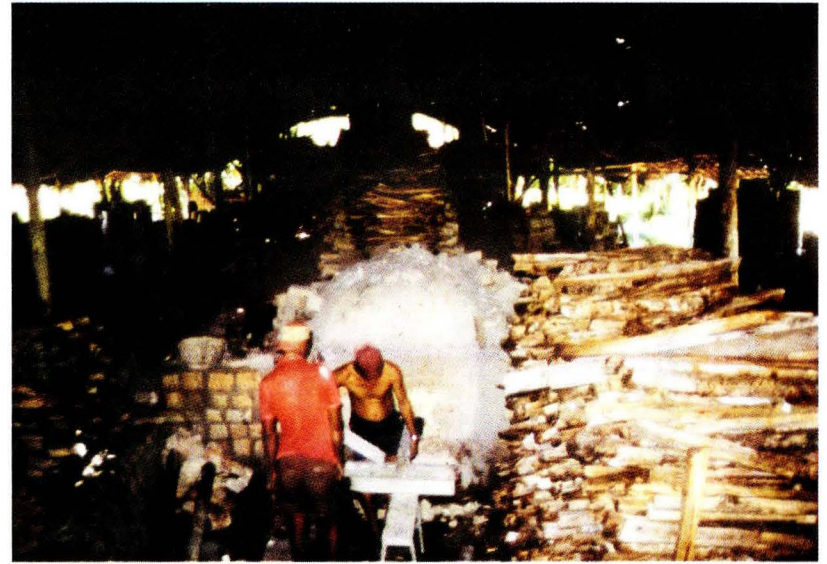
34. Pembersihan dan pengecekan tungku sebelum pembakaran Cleaning and checking the kiln before firing
