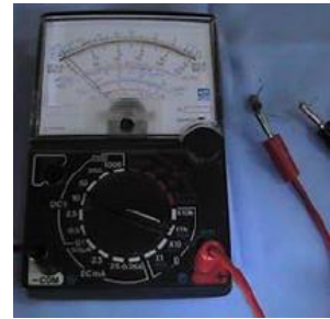
Gambar 1.97. Pengetesan basis emitor reverse
