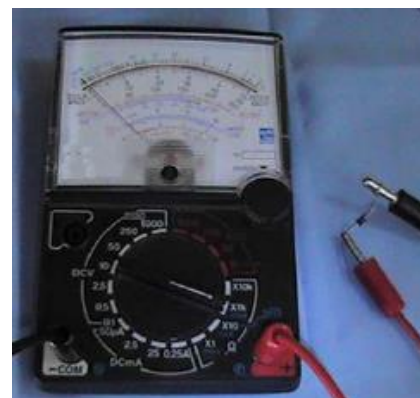
Gambar 1.91. Pengetesan dioda bias balik
