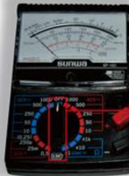
Gambar 1.53. Fungsi selector switch
