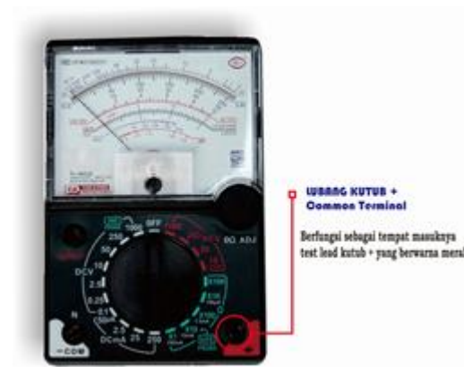
Gambar 1.55. Fungsi lubang kutub+(common terminal)
