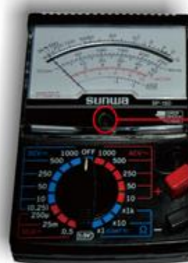
Gambar 1.51. Fungsi zero adjust screw
